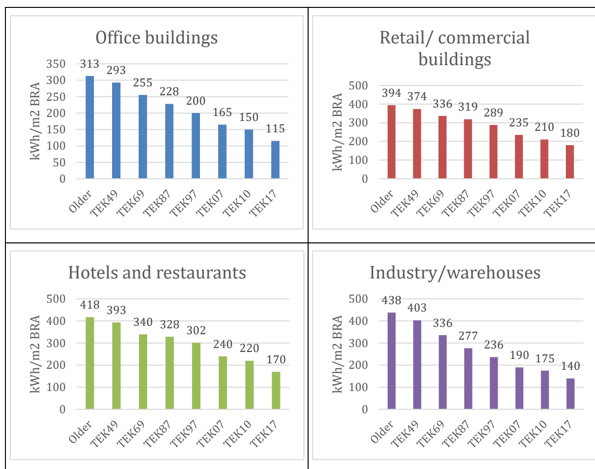
Figure 13 Development in calculated specific net energy demand based on building code and building tradition (Multiconsult, simulated in SIMIEN)
