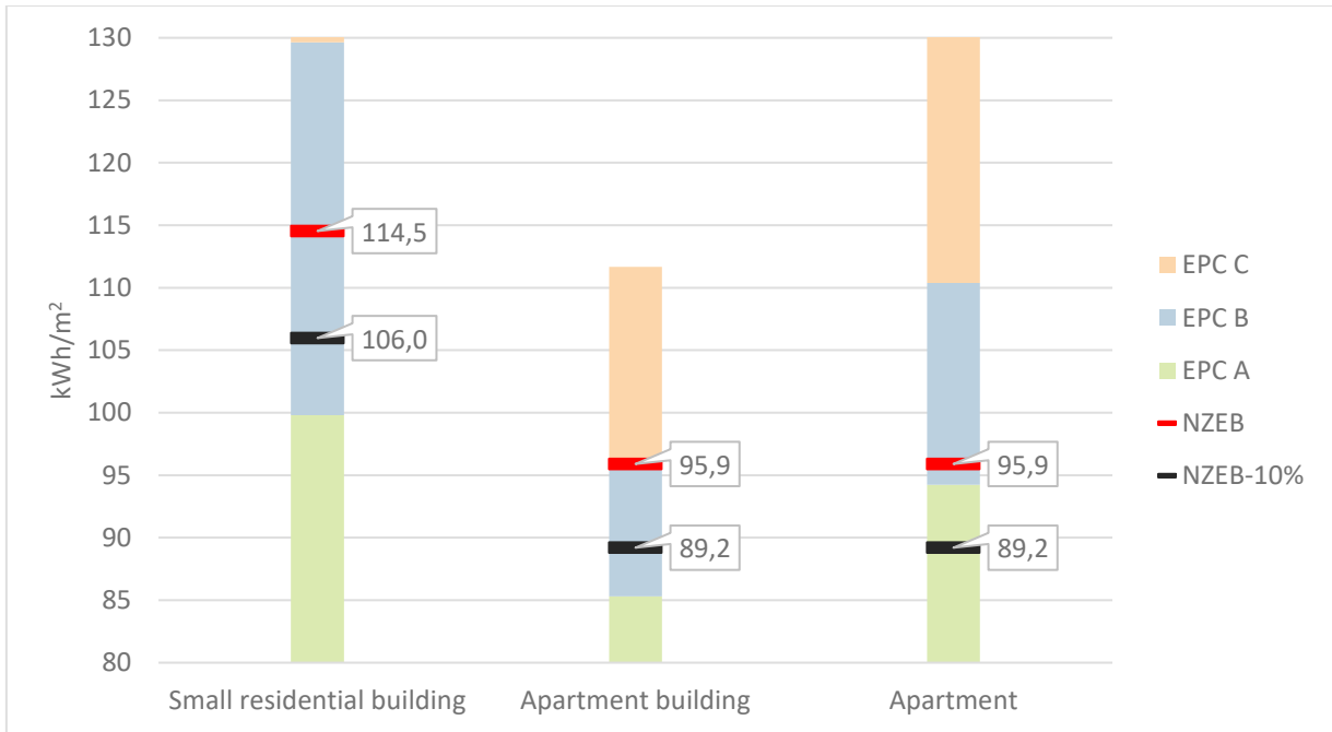
Figure 2 Energy performance with reference to the national definition of NZEB and NZEB-10 percent compared to limit values in the EPC system (values dependent on dwelling area).
